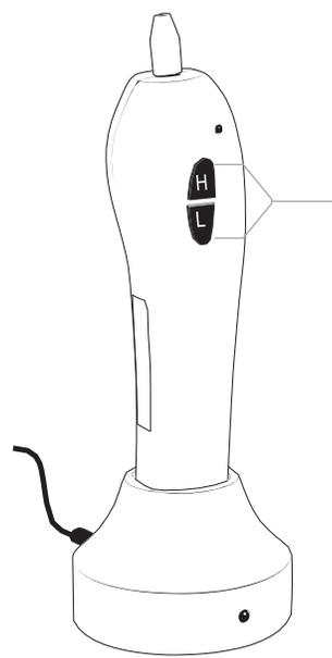
On the device, there are two buttons used to provide two different output voltages, marked with inscriptions "H" high and "L" low.
